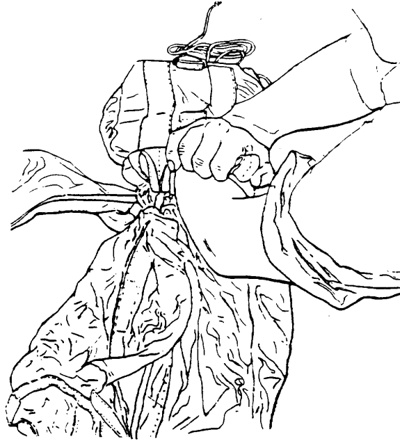
Figure 22. S-Folding the Canopy.
